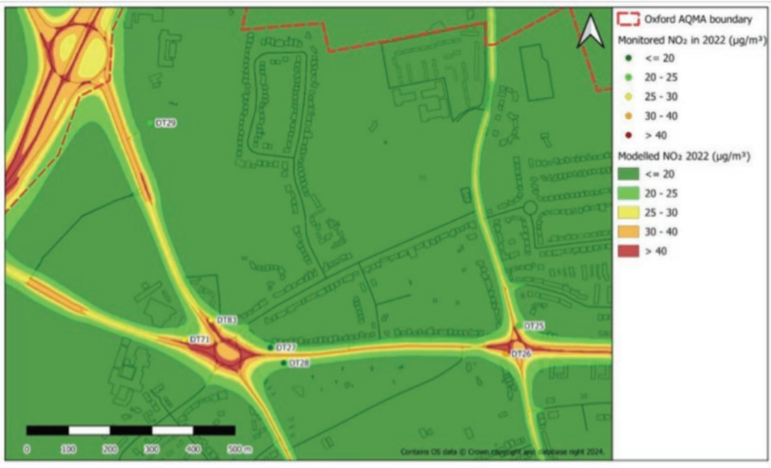
Figure 19 - Baseline model results and measured NO 2 in 2022 near Cutteslowe Roundabout.
